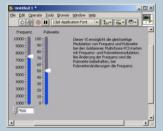
Display of the control inputs: Frequency and pulse width are adjusted by the sliders.
